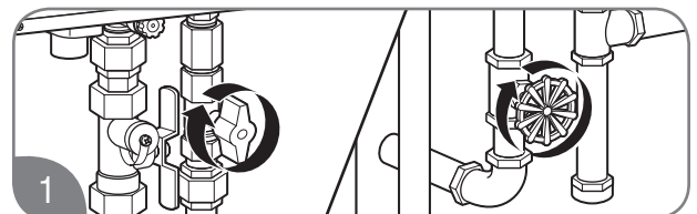
1 Turn off the gas and water to the water heater by closing the shut-off valves.
