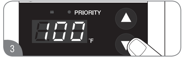
3 Press the DOWN adjustment button repeatedly until 100°F (38°C) shows in the LED display.
