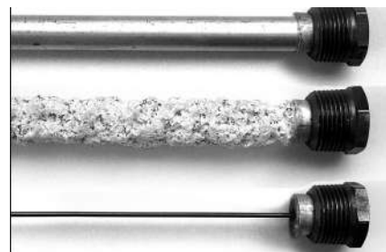
Figure 27 - Anode Rods from new (top) to partially depleted (middle) to fully depleted stage (bottom)
