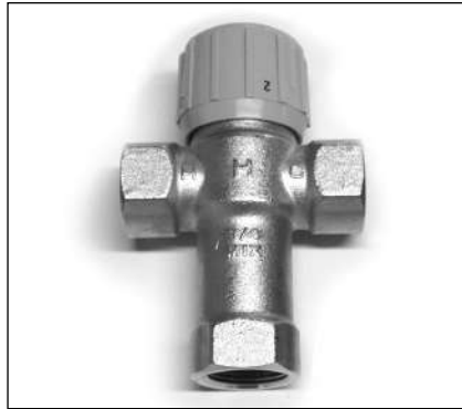
Figure 20 - Adjust Thermostat Mixing Valves at each point-of-use 120°F or lower.
