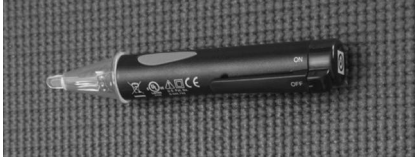
Figure 2 - Use a non-contact circuit tester to insure that the power is off before you work on a circuit.
