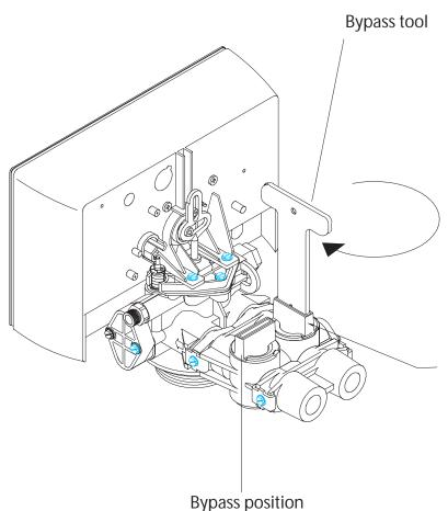
Use the bypass tool to turn the valve handles from service to the bypass position
