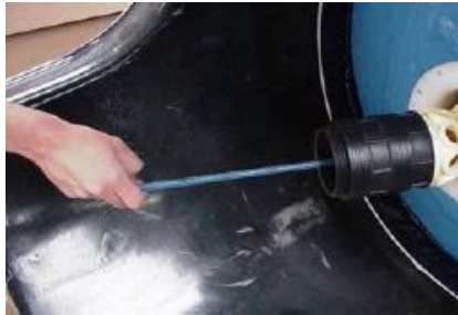
Step 2: Parts shown in Step 1 are assembled (outside of tank) and inserted in tank using extension I-WR03-LA.
