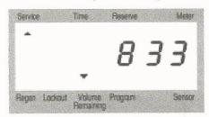
For Example: 833 Gallons Of Water Remaining (Valve in Service)
