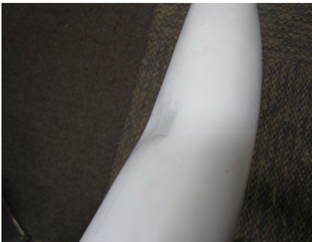
Figure 1. Defect: Small Dent
