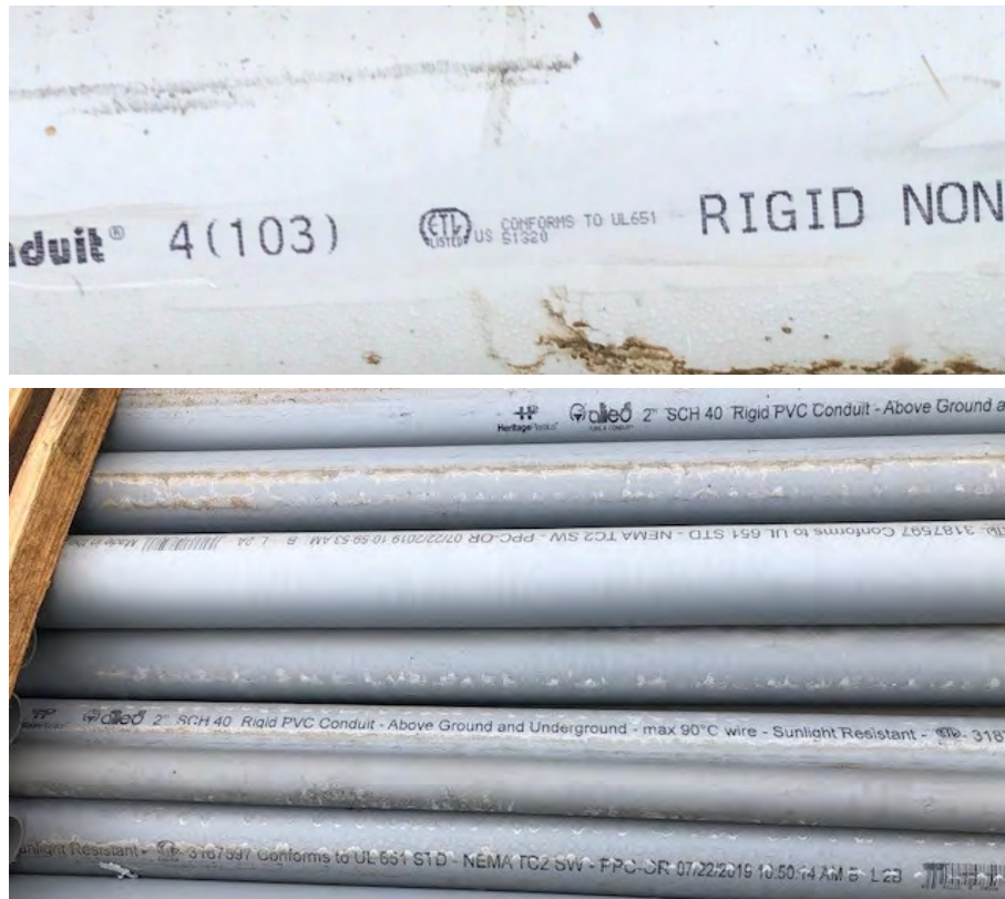
Figure 5. UL 651 or ETL Conforms to UL 651 Marking
