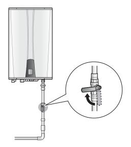
5. Open all hot water faucets completely. The water that remains in the plumbing lines will drain out.
