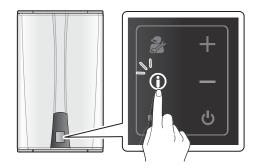
Press the + or - buttons to switch between the information types.
