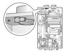
5. Pull the filter out of the water heater.
