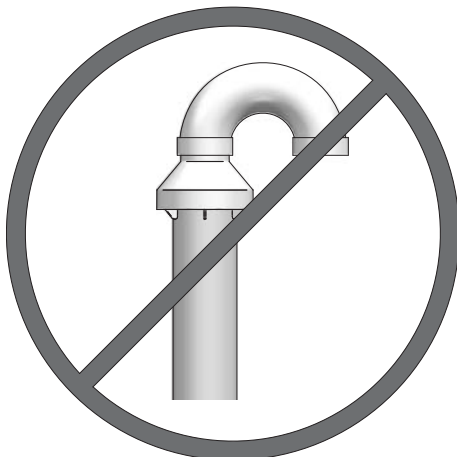
Figure 4-5 Do Not Install U-Bent to Rain Cap
