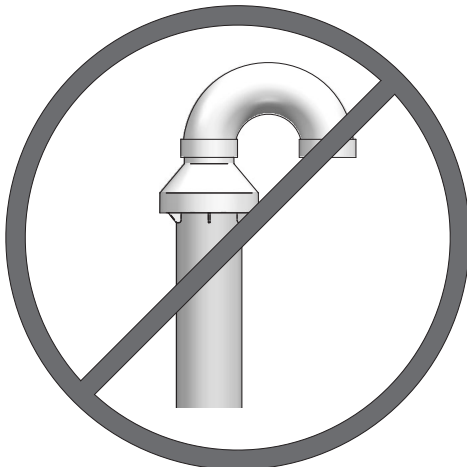
Figure 5-5 Do Not Install U-Bend to Rain Cap
