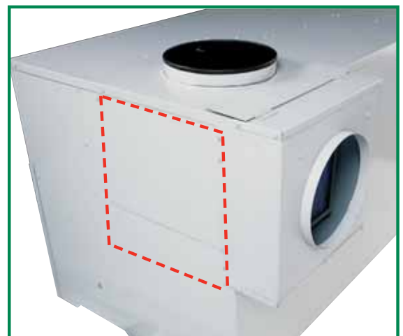
For easier and more flexible installation the air inlet box is field convertible mounting on either the rear or side of the unit. With this feature the unit can be direct vented with up to 50 equivalent feet of air inlet and 50 equivalent feet of outlet vent and does not require the same pressure zone for inlet and outlet locations.
