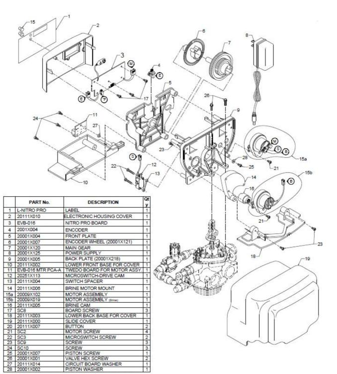
LETTERS IN DIAGRAM REPRESENT WIRING CONNECTIONS
