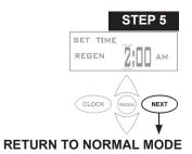
STEP 5 – Next Regeneration Time (minutes): Set the minutes of day for regeneration using or buttons. Press NEXT to return to normal operation. Press regeneration to return to previous step.
