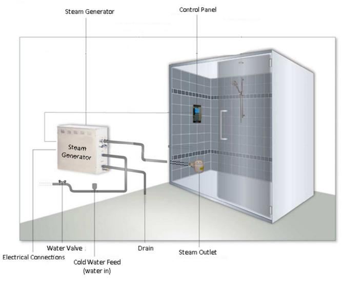
Above is the typical set up for installing your steam generator kit, however models do vary, but the actual set up is always similar.
