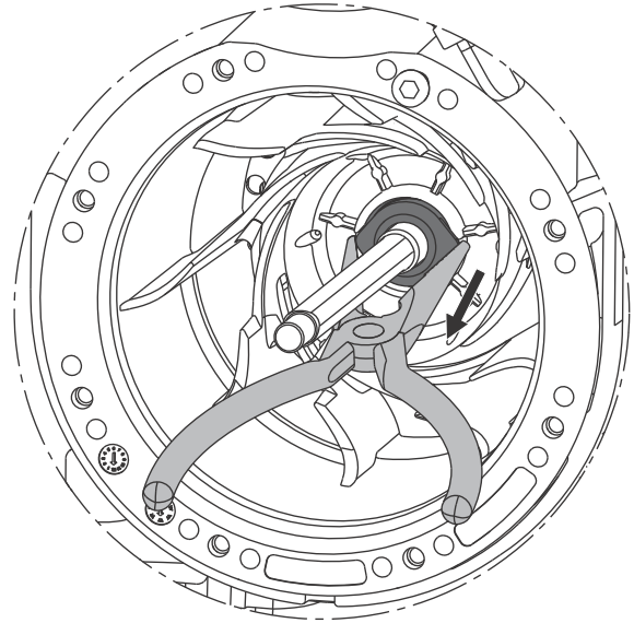
Fig. 12 Removing the stationary shaft seal
