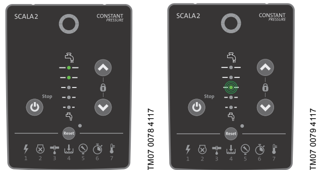
Fig. 18 User-defined setpoint (left) and self-learned setpoint (right)
