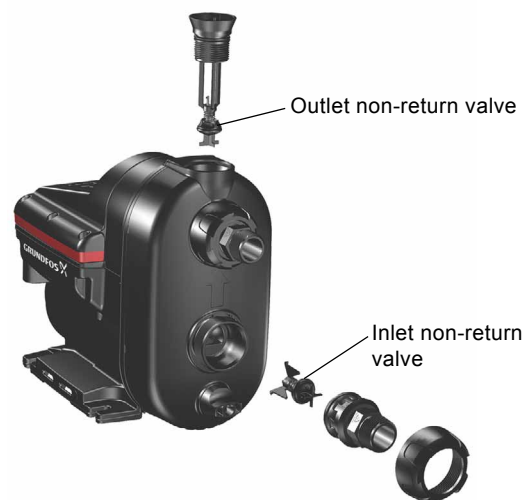
Fig. 20 Outlet and inlet non-return valves
