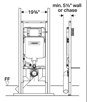
RH, LH or vertical drainage runs allowed with 5 1/2" minimum wall thickness.
