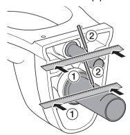
Add dimension X and 1/8". Using that dimension, mark a line on the pipe measuring from the hub side. Cut off the pipe at the line with a pipe cutter.
