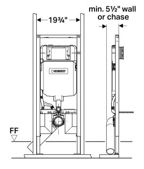
RH, LH or vertical drainage runs allowed with 5 ½" minimum wall thickness.
