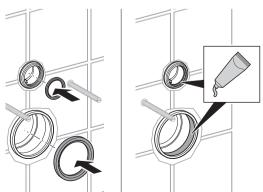
Remove protective sleeves from mounting rods. Determine protruding rod length for bowl installation. Install both pipes into the hubs in the wall.
