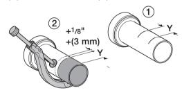
6 Bevel the sharp edges as shown to assure a smooth insertion into the pipe hubs in the wall.
