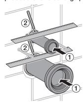
Place discharge pipe with gasket into waste outlet of bowl. Also place flush pipe with fin gasket into inlet of bowl. Then mark a second line on both pipes.
