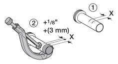
Add dimension Y and 1/8". Using that dimension, mark a line on the pipe measuring from the hub side. Cut off the pipe at the line with a pipe cutter.
