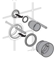
2 Insert discharge pipe into the pipe hub in the wall. Place a straight edge flush against the wall and mark a line on the pipe. Fit finned rubber seal onto flush pipe. Repeat same procedure for discharge pipe.
