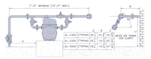
Typical 1400, 2300, and 5000 Meter Fit Installation for Low Gas Pressure Delivery.
