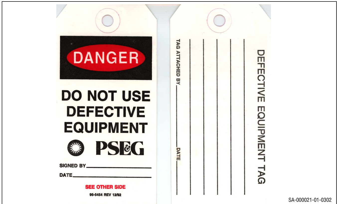
Figure 7.1: Defective Equipment Tag (PSE&G Form 95-5454)
