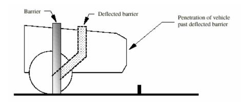
This type of collision is called an inelastic collision, where the momentum (p) of the vehicle equals the momentum gained by the bollard, as shown in the following equation.
