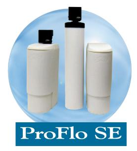
Elite® Proflo SE Series' control is designed to meet today's higher flow demands, reducing pressure drop across the system. The Proflo SE control is demand initiated by a compact turbine meter which monitors water usage. It incorporates fully adjustable electronics to adjust to specific water problems and upflow brining for increased salt and water savings during regeneration.
