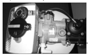
Attach meter cable into meter assembly.
