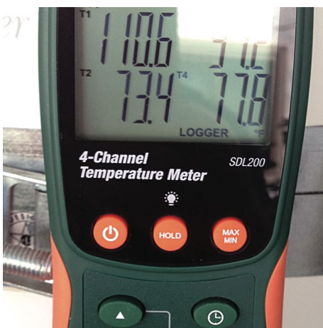
Figure 4. Extech SDL200 4-Channel Temperature Meter and Data Logger. Logging interval set to 10-seconds for 48+ hours captured essential data for forensic analysis.
