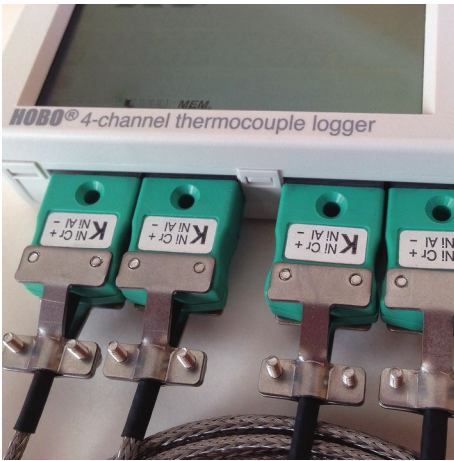
Figure 5. The UX120-014M provides four dedicated thermocouple channels and an internal ambient temperature sensor.
