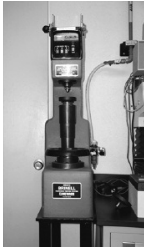
Figure 26—Brinell Hardness Tester: Tests the Hardness of Cast Iron. Additional Quality Control Testing Performed by CISPI Members Not Required by CISPI or ASTM Standards.
