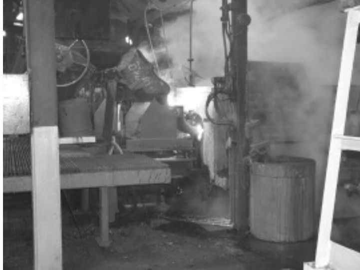
Figure 7—Iron being poured into spinning pipe mold.
