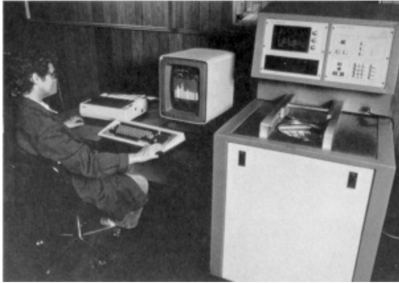
Figure 21—Energy Dispersive X-Ray Spectrometer: Analysis of Iron, Slag, and Raw Materials.
