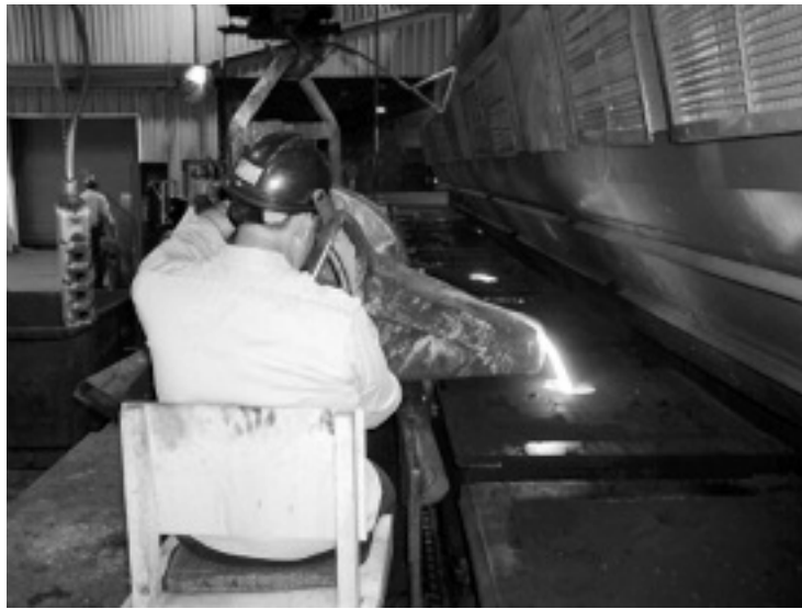
Figure 14—Hand-Pouring of Cast Iron Soil Pipe Fittings.
