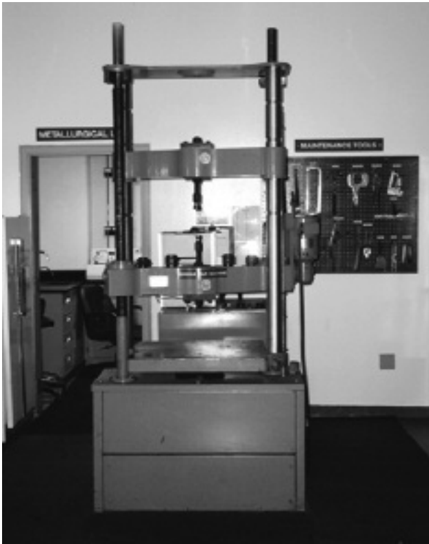
Figure 25—Tensile Tester: Tests Tensile Strength of Cast Iron Test Bar. 21,000 psi Minimum, Required by CISPI and ASTM Standards.
