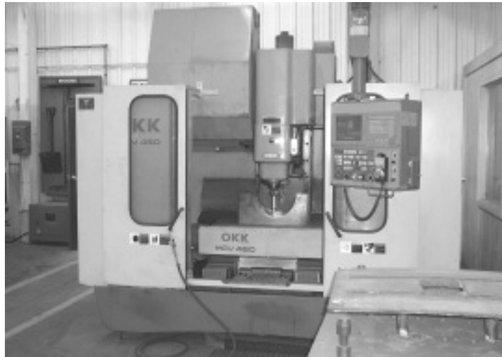
Figure 9—Operation of Precision Milling Machinery for Patternmaking.
