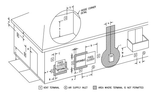
Figure 1 - Vent Terminal Clearances
