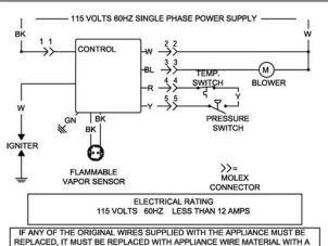
MINIMUM TEMPERATURE RATING OF 105°C AND A MINIMUM SIZE OF NO. 18 AWG. Figure 6
