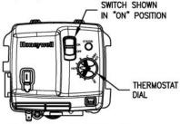
5. Slide the switch on the right side of the gas valve down to the "OFF" position
