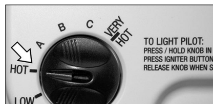
Figure 36 - Adjust the gas control knob to "HOT".
