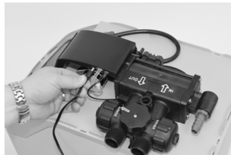
Diagram 14: Connect Transformer Power Cord
