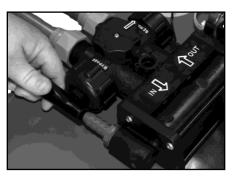
Figure 5: Connect Drain Line
