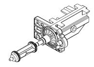
Rotate The Piston Assembly 90 Degrees Clockwise Until You Hear An Audible Click As It Snaps Into Place
