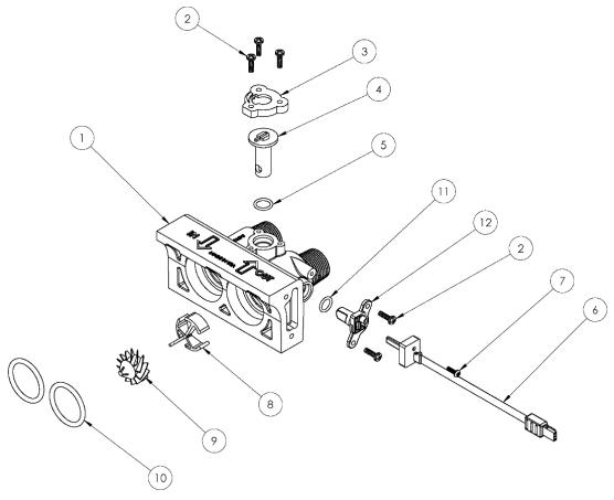
Figure 18: Optional 3/4-inch (19-mm) I/O Adapter Assembly with Blending Valve
