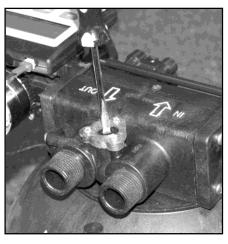
Figure 10: Adjusting Blending Valve
