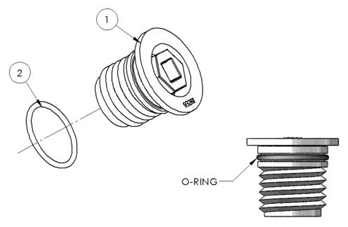
Figure 19: Top Fill Plug Assembly
