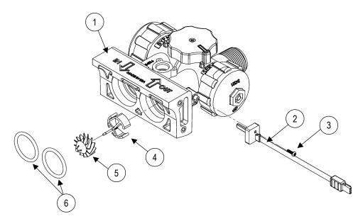
Figure 17: Bypass Valve Assembly
