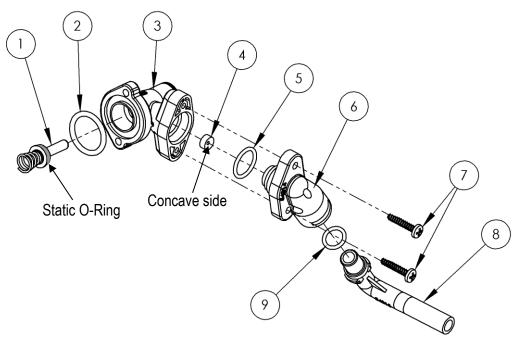
Figure 22: Brine Valve Housing Assembly
