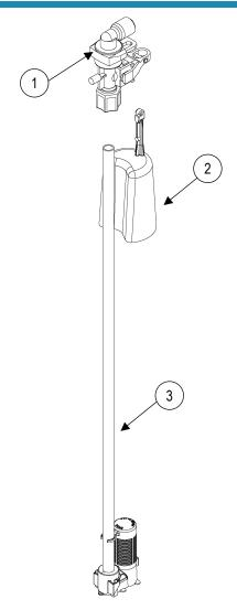
Figure 23: Safety Shutoff Assembly
