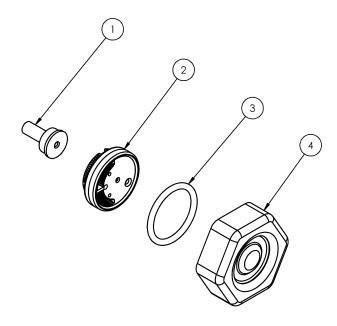
Figure 16: Injector Assembly
