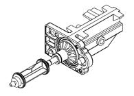
Slide Piston Assembly Onto Piston Slide. Push Toward End Cap To Stop.
