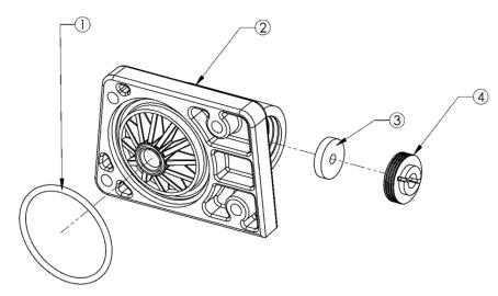
Figure 20: Drain End Cap Assembly
