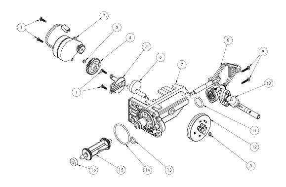
Figure 21: Drive End Cap Assembly
