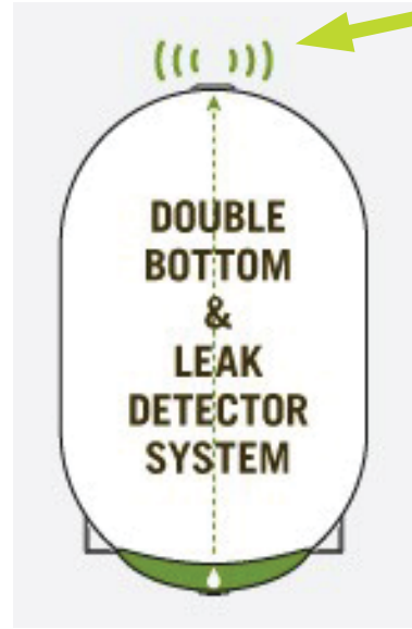
This drawing illustrates the structure of a double bottom tank. The area most subject to corrosion is the tank bottom. These tanks are fitted with an inspection port which allows you to see if the tank has failed.
