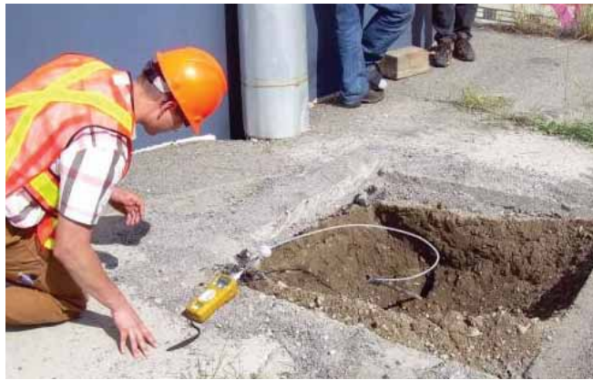
Engineer testing level of contamination in the soil.
