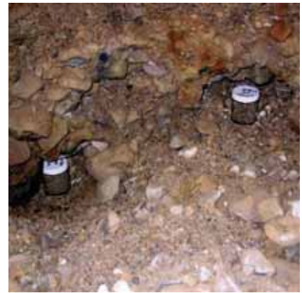
Sample bottles prepared for testing lab to determine parts per million of oil in contaminated soil.
