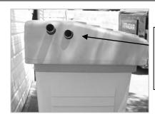
Cut holes with hole saw ½" larger than piping.
