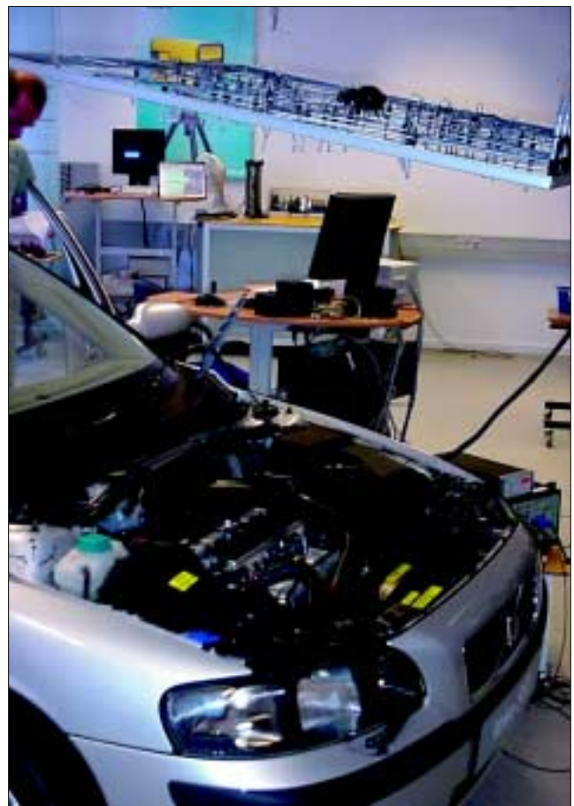
Figure 33. Beamformer placed above an engine.
