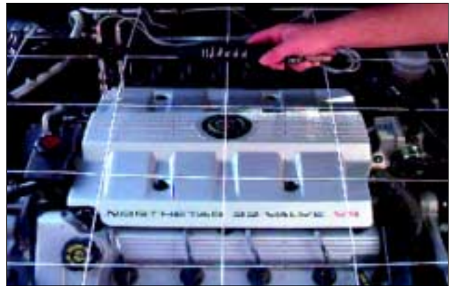
Figure 4. Sound intensity measurement procedure on a car engine.
