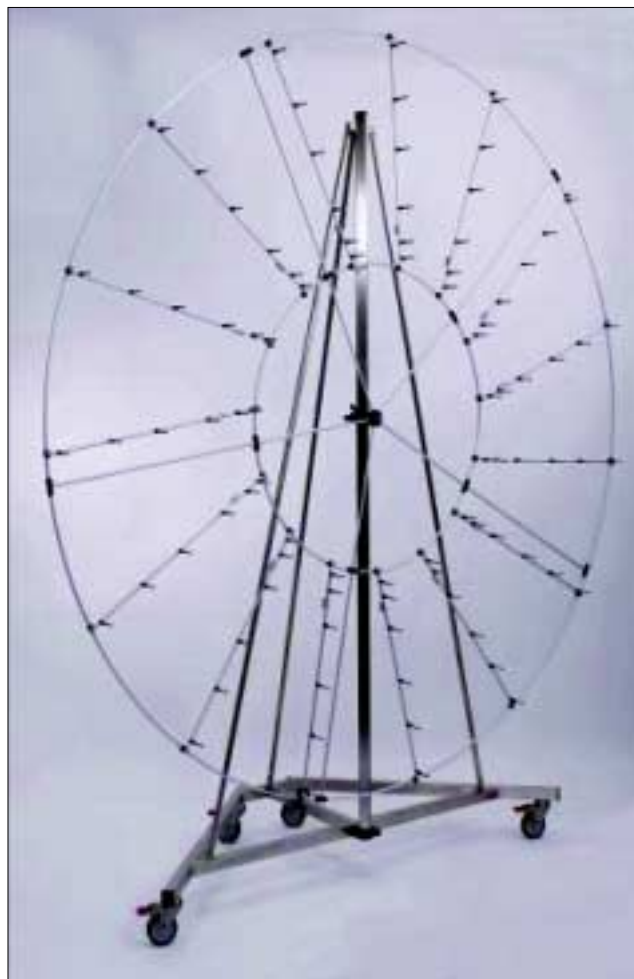
Figure 31. Example of a 90-channel Brüel & Kjær wheel array for beamforming. The wheel array depicted has 15 identical spokes with integrated cabling each carrying 6 microphones. The wheel diameter is 2.43 m (patent pending).
