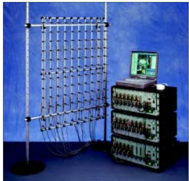
Figure 17. NS-STSF technique, full-sized microphone array.
