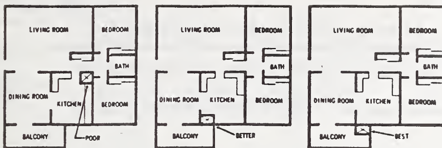
Selecting proper location of closet-installed furnace unit.
