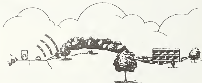
FIG. 6-3 ACOUSTICAL SHIELDING PROVIDED BY LANDSCAPE AND NATURAL AND MAN-MADE BARRIERS.
