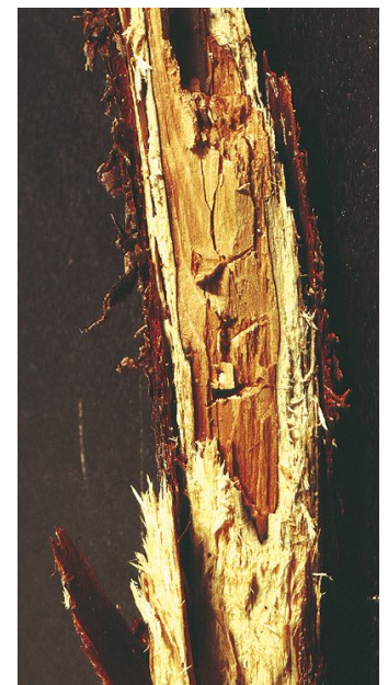
Figure 1. Dead, decaying stem with white rot in the outer wood and brown rot in the inner wood caused by two different fungi. The white rot is stringy-fibrous; the brown rot breaks easily across the grain, has no fibrous strength, and is crumbly when dry. Photo: Jim Worrall, USDA Forest Service.
