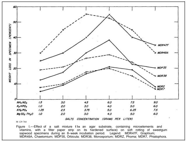
increased soft-rot attack. An example of the advantage of using the nitrogen, phosphate, and magnesium medium is shown in figure 1. In the experiment on which the figure is based, specimens of sweetgum sapwood were laid on a square of filter paper resting on the agar. The rate of soft rot was maximum when the concentrations of salts, in grams per liter, were 6 of  $NH_4NO_3$ , 4 of  $K_2HPO_4$ , 5 of  $KH_2PO_4$ , and 4 of  $MgSO_4$ ·7 $H_2O$ .
