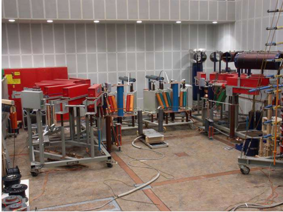
Fig. 17- Example of an impulse current generator
