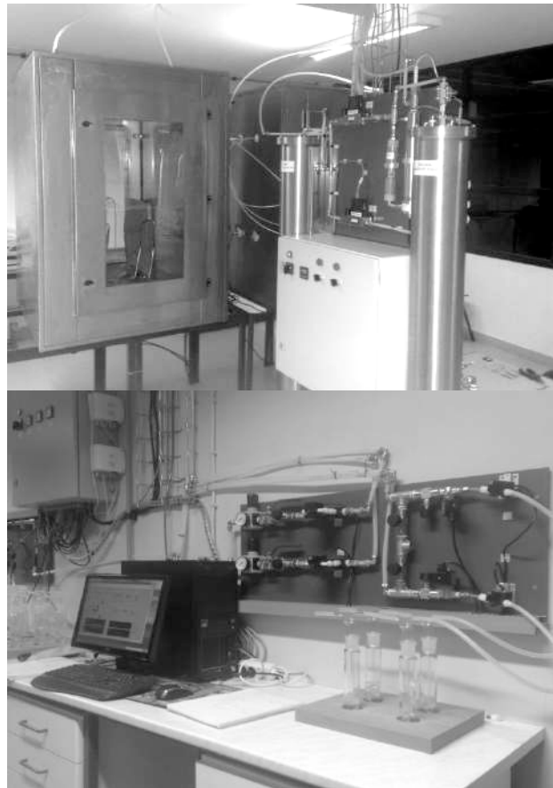
Figure 4.2. Images of small chamber method implementation. Left: 1 \text{ m}^3 chamber according to EN 717-1 and air cleaning and conditioning system. Right: gas sampling system.
