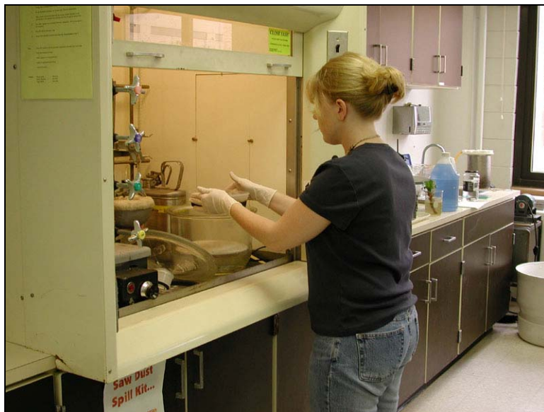
Figure 39. Placing Linoleum #6 in Vacuum Chamber (photo by E. Eilert)
