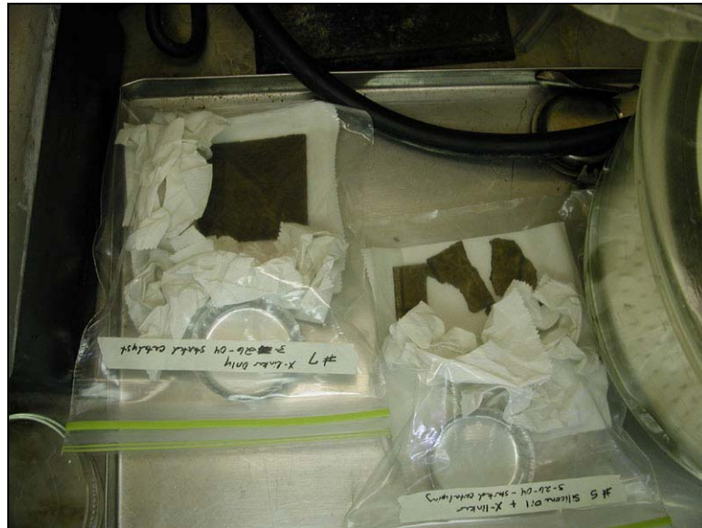
Figure 42. Linoleum #7 In Fume Hood Going Through Catalyzation Process (photo by B. E. Coke)
