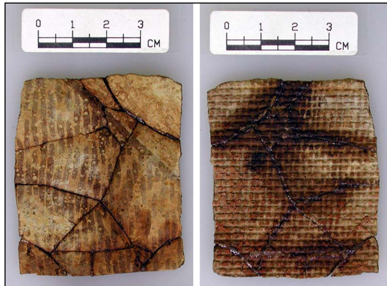
Figure 48. Post Treatment Image of Linoleum #2 with Re-glued Sections (photo by B. E. Coke)
