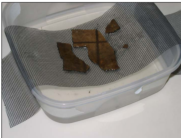
Figure 35. Linoleum #5 Draining on Mesh Screen (photo by B. E. Coke)
