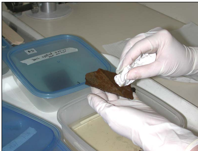
Figure 32. Wiping Excess Solution off Linoleum #4 (photo by E. Eilert)
