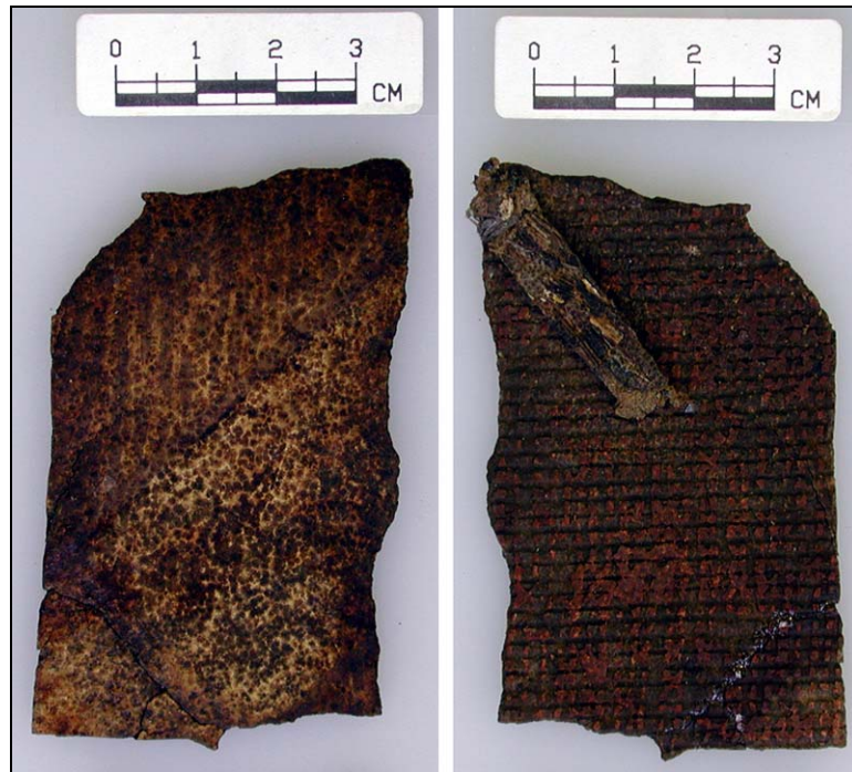
Figure 50. Post Treatment Image of Linoleum #4 with Re-glued Sections (photo by B. E. Coke)
