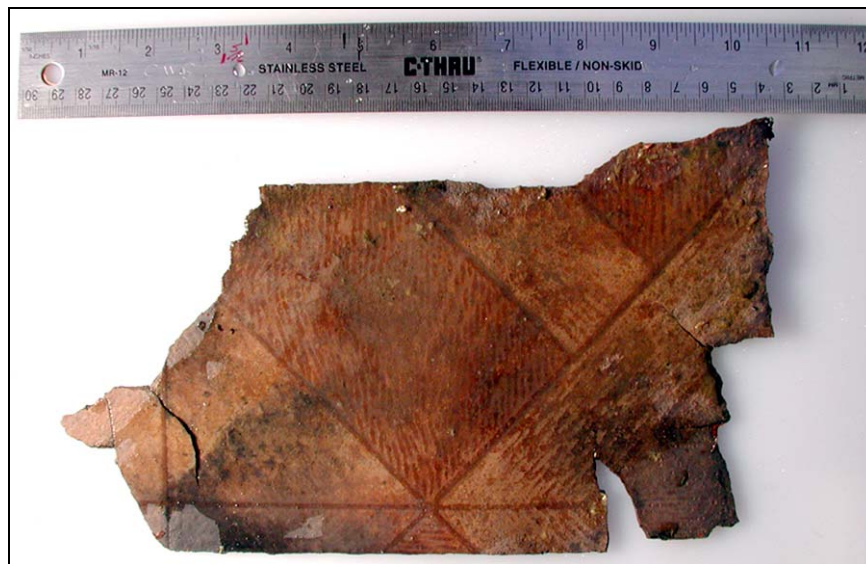
Figure 11. Linoleum Sent to APRL for Conservation (photo by B. E. Coke)
