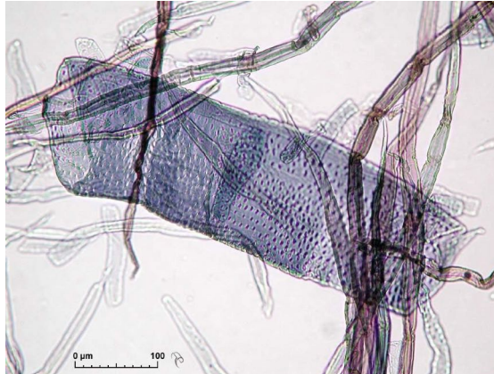
Vessel element with an optimum view of its pits (Photo kindness: Econotech Services Ltd.)
