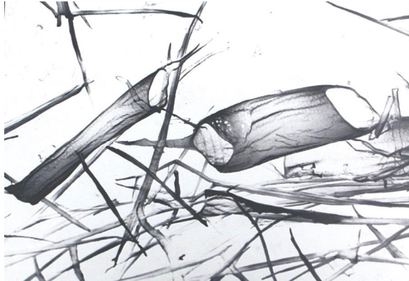
Eucalyptus vessel elements shaped as glazed clay pipes or little barrels
