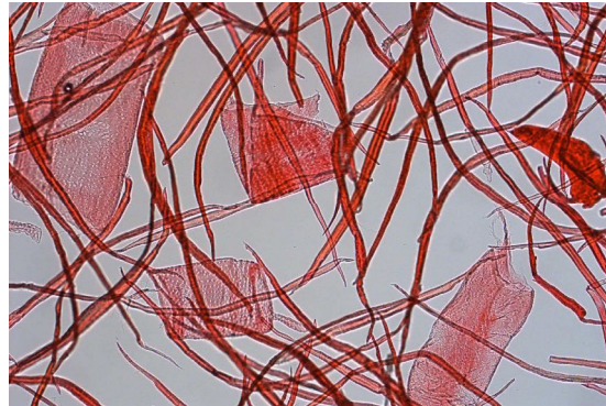
E. globulus pulp – vessel element rich fraction, obtained by hydrocyclone fractionation (Source: Panula-Ontto, 2007)
