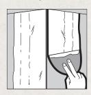
Using a 6" taping knife for outside corners (4" for inside corners), apply another coat of joint compound (USG Sheetrock® Brand Easy Sand™, Topping, All Purpose, or Lightweight All Purpose). Keep this coat as smooth as possible. Feather out 5" to 6" (125 to 150 mm) from the nose of the trim on each side for outside corners (1" or 25 mm past previous coat for inside corners). Let dry. Sand sides lightly where needed.
