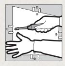
d. Remove tabs from each drywall repair clip. Apply compound and tape to all four section sides. Do not overlap tape. Apply second and third coats of joint compound, allowing each coat to harden before applying next coat and feathering out from previous coats. Sand and prime when dry.
