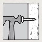
Double-nailing reduces the likelihood of nail pops. It is highly recommended for ceilings. Drive first nails 12" o.c. along framing in the field of the board and second nails about 2" from the first. Fasten the perimeter 7" o.c. for ceilings and 8" o.c. for walls.
