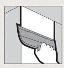
Allow third coat to dry overnight (drying time may vary, depending on temperature, humidity and jobsite conditions). Lightly sand imperfections in finished joints, corners and over fastener heads. Carefully remove sanding dust with damp sponge. Use a dust collection with a HEPA filter with power sanding. Wear a dust mask if excessive dust is produced and the area cannot be ventilated.
