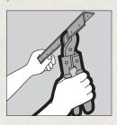
Force bead onto corner being careful that the flanges don't spread beyond 90° angle, making it hard to cover them with joint compound.
