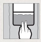
Apply a 7"-8" coat of joint compound to each side of butt joints and feather. Compound should extend beyond first coat for a total width of 14".
