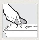
Keep the blade clean, especially of dried bits of compound, to avoid leaving scratches in the wet joint compound as you draw the knife over it. Discard any compound containing dried bits of material. Clean blade by drawing it over edge of pan.
