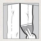
Use an 8" or larger finishing knife for outside corners (4"-6" knife for inside corners) to apply a finishing coat of the same ready-mixed or setting-type compound. Feather compound 8" (200 mm) from nose of trim for outside corners (1" [25 mm] past previous coat for inside corners). Let dry. Sand and prime.
