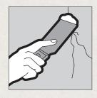
c. To repair a popped nail, drive and dimple new nail 1-1/2" from popped nail. Drive and dimple popped nail. Cover with joint compound. Sand and prime when dry.
