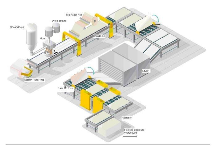
Gypsum, the main raw material, comes from one of four sources: DSG is transported from power stations, natural gypsum is extracted from mines and quarries, process scrap is reformed into new product and construction / demolition waste is collected from jobsites and returned to the plant for reprocessing. This material is calcined before use to produce the hemihydrate of calcium sulphate – stucco (CaSO4•1/2 H2O). This stucco is stored in silos.
