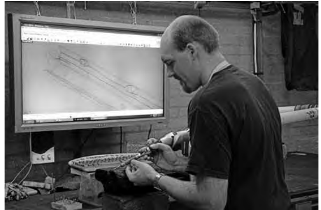
Fig. 44.2. Recording a ship's timber using FaroArm and Rhino software (Photo: © Newport Museum and Heritage Service).
