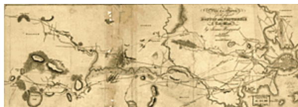
Right Half of James Hayward's 1828 plan of a survey for the proposed Boston and Providence Railway. This is the earliest topographic strip map in the Library showing a railroad survey. These lines were originally intended for horse drawn trains.
