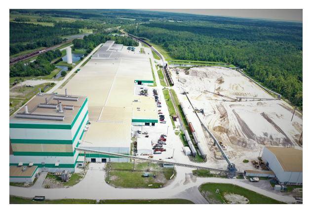
Saint-Gobain, through its building products subsidiary CertainTeed LLC, will install recycling technology at its gypsum plant in Palatka, Florida, increasing the recycled content in its wallboard products manufactured in Palatka by 18,000 tons/year while also reducing the site's carbon dioxide emissions by 2,260 tons/year.
