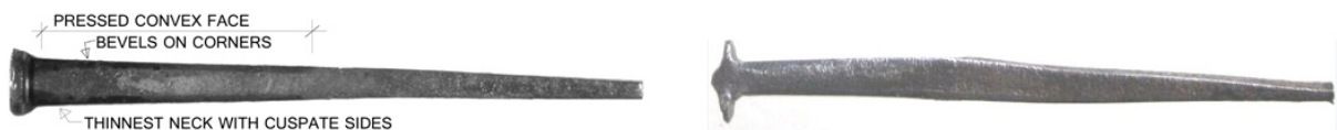
Fig. 5. An American ‘fine’ face-clamped cut nail of 1877 from Warrnambool & a British side-clamped cut clasp nail of circa 1856 from Coleraine. Author.
