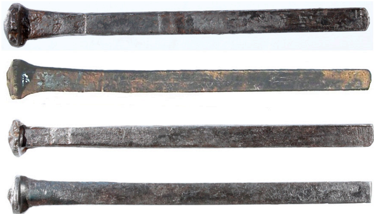
Fig. 3. Wrought forms of Ewbank nails; 1836, 1869, 1881 and the cut form facsimile T-patent of 1870. Author.
