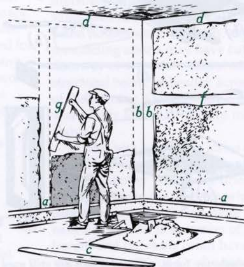
Cornerite is installed at all the interior angles.
