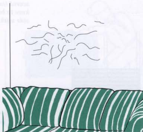
Map cracking, named for its resemblance to a crumpled map, indicates that the surface finish coat of plaster is pulling away from the basecoat.
