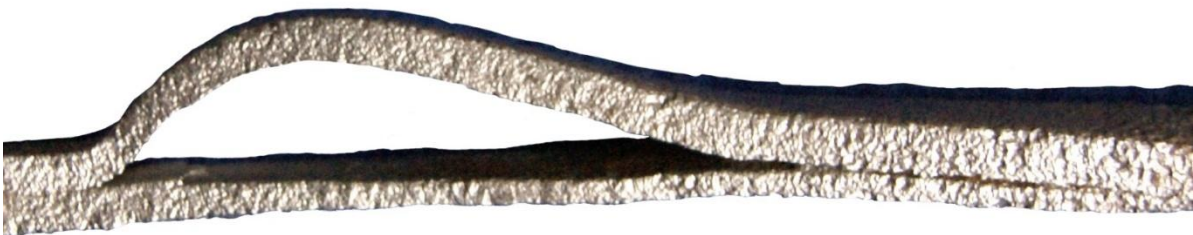
Figure 7 – The corbel and de-bonding towards the head
