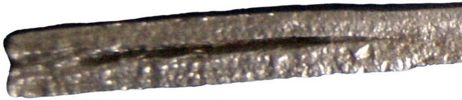
Figure 8 – De-lamination of fibres at tip
