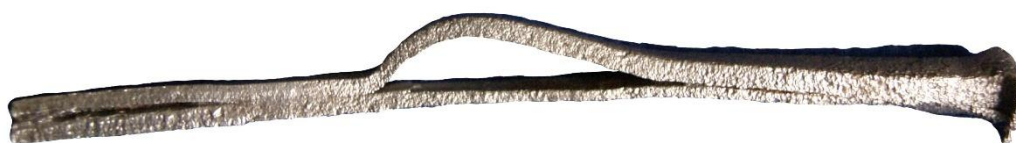
Figure 5 – The nail showing corbel and de-bonding of fibres
