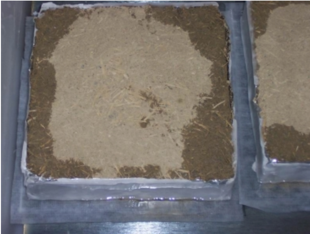
Figure 5.5: Water wicking at edges
