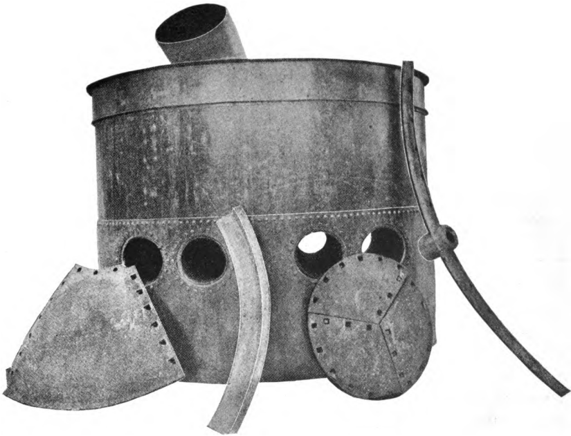
Four-flue kettle for calcination of gypsum
