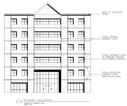
Figure 4.2.5 – Typical location of movement joints on a direct adhered facade.
