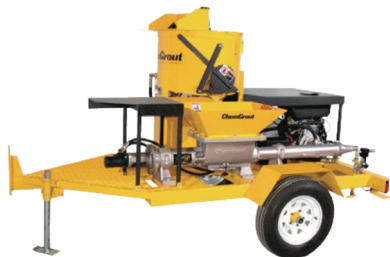
Figure 5.3.2 — Sprayer/Pump for cementitious plasters/renders. Example shown: ChemGrout CG-575 Series Thick Mix Sprayer/Pump — Trailer Mounted. Max. output 2 — 8 GPM; max pressure 261 psi (18 bars). Material and job versatile. Mixes and pumps or sprays thick to thin materials including repair mortars, gel mortars, grouts, plasters, stucco, EIFS, fireproofing, cement/sand, cement/fly ash, flowable and non-flowable grouts, Bentonite waterproofing grouts.
