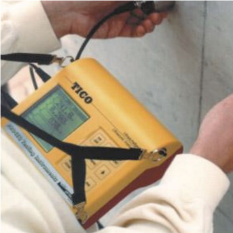
Figure 9.4.3— Ultrasonic pulse velocity equipment. 19
