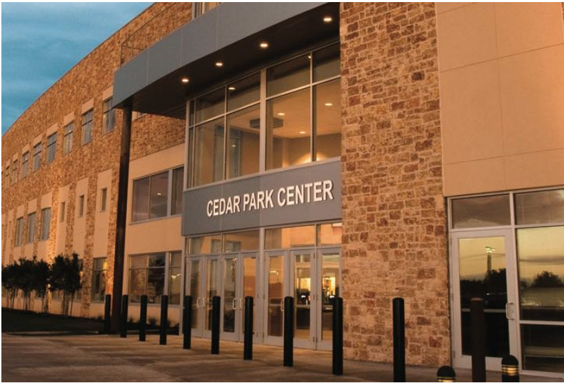
Photo: Project — Cedar Park Center, Cedar Park, TX; Contractor: Trinity Drywall & Plastering Systems Fort Worth, TX. Description: Limestone and Sedona Red Flagstone façade installed with MVIS™ Air & Water Barrier and MVIS Veneer Mortar.
