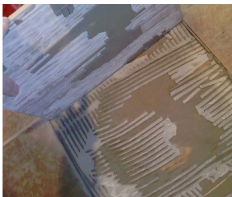
Figure 7.4.10 — Improper beat-in or vibration results in no contact with adhesive.
